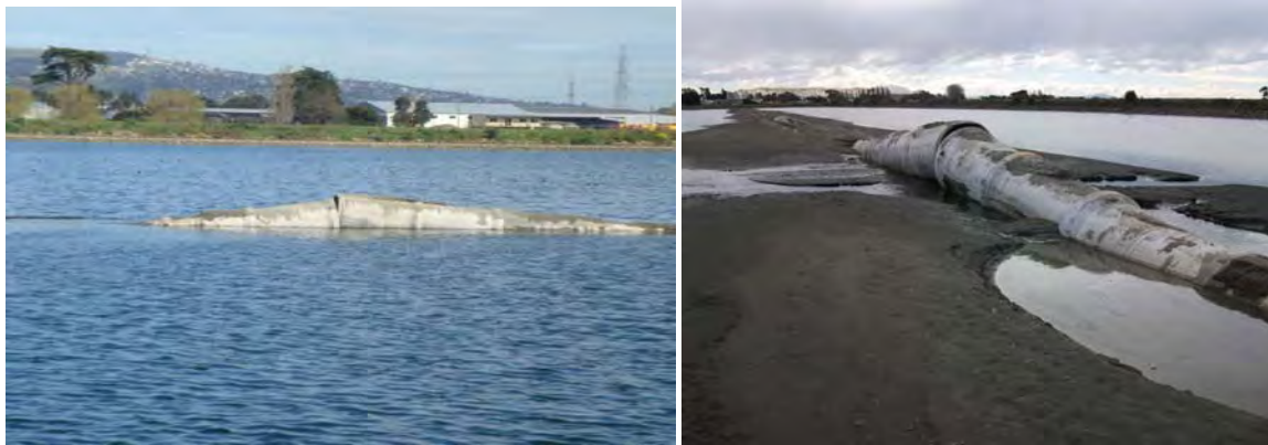
Figure 6.34 Buckled pipe protruding from Pond 1 during pond dewatering, and after pond level was lowered. Pipeline crown was at the pond invert prior to the earthquake. (-43.530867°, 172.705190°)
