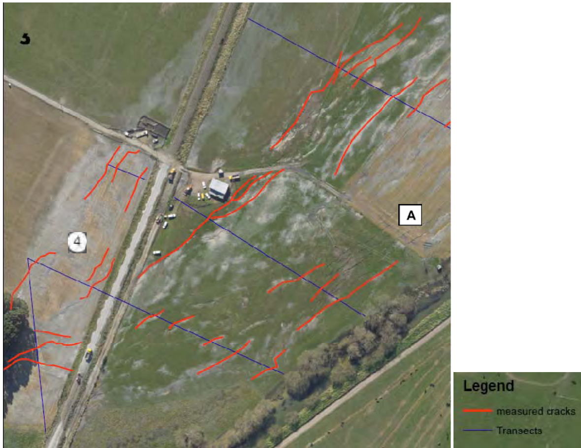
Figure 4.31 Aerial view of the lateral spreading area at position A at South Kaiapoi showing four transects of detailed ground surveys.
