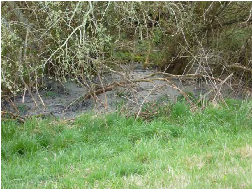
Figure 6.8 Photo 3: Liquefaction ejecta (center of photo) along the base of the levee on Coutts Island Rd (riverside). The location of this photograph is denoted in Figure 6.4. ( -43.424093^{\circ} , 172.630468^{\circ} )
