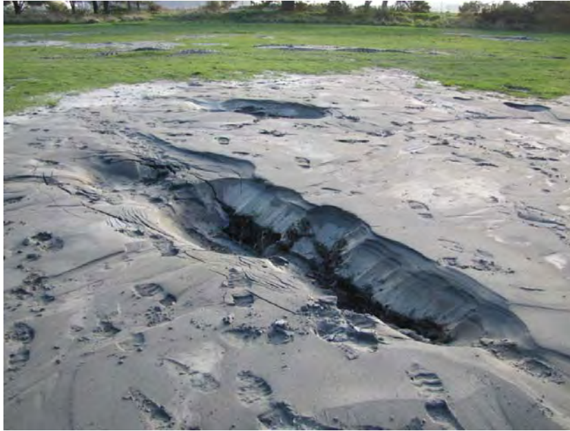
Figure 4.14 Sandboil in the Featherstone Reserve Pines Beach from which sand was taken for electron microscope pictures. (Approximate position: -43.381111^{\circ} , 172.703611^{\circ} )
