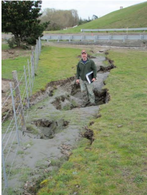
Figure 7.25 Evidence of liquefaction adjacent to Chaney's Overpass. ( -43.4300^{\circ} , 172.6464^{\circ} )
