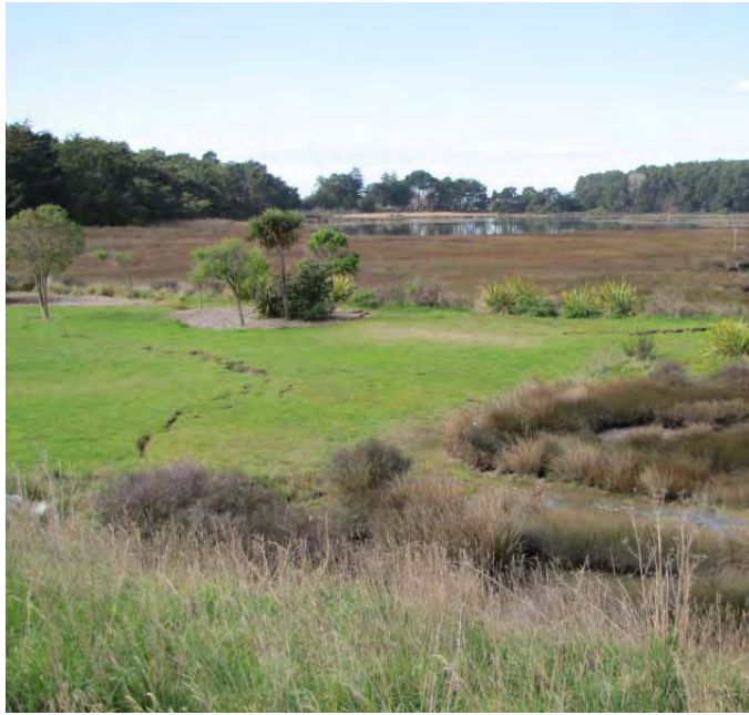
Figure 7.3 Lateral spreading of east banks adjacent to the Bridge Street Bridge. ( -43.5253^{\circ} , 172.7242^{\circ} )
