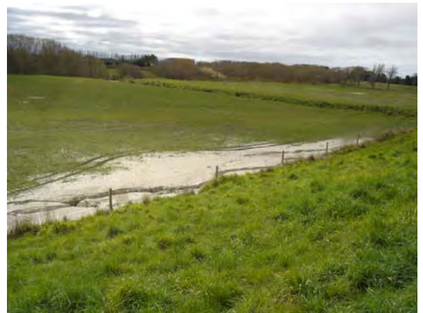
Figure 6.18 Photos 11 - 14: Liquefaction ejecta on both the river and landsides of the levee. The locations of these photographs are denoted in Figure 6.4. ( -43.428968^{\circ} , 172.645435^{\circ} )
