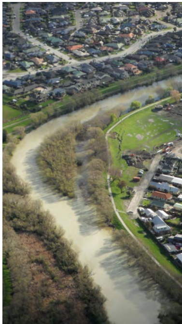
Figure 6.24 Photos 23 and 24: Aerial photographs of lateral spreading of levees on the north bank of the Kaiapoi River. The locations of these photographs are denoted in Figure 6.4. (left: -43.387389^\circ , 172.666173^\circ ; right: -43.386875^\circ , 172.672297^\circ )
