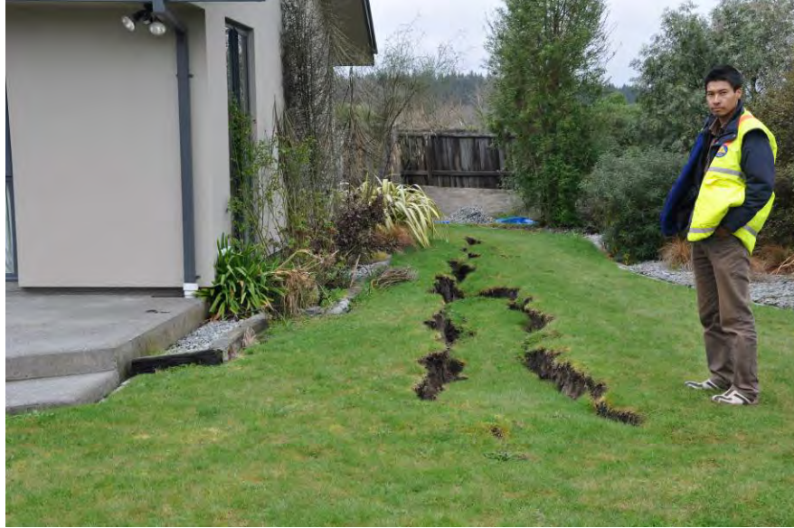
Figure 5.46. Lateral spread adjacent to residence at Riverside Ln. The location of this fissure is ~26 m from the nearby Styx River. ( -43.4308^{\circ} , 172.6930^{\circ} ; 1230 hrs on 13 September 2010)
