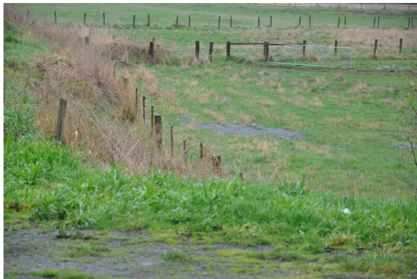
Figure 7.34 Evidence of liquefaction in surrounding low lying marshlands on the east side of the Kainga road bridge ( -43.3995^{\circ} , 172.6917^{\circ} ).
