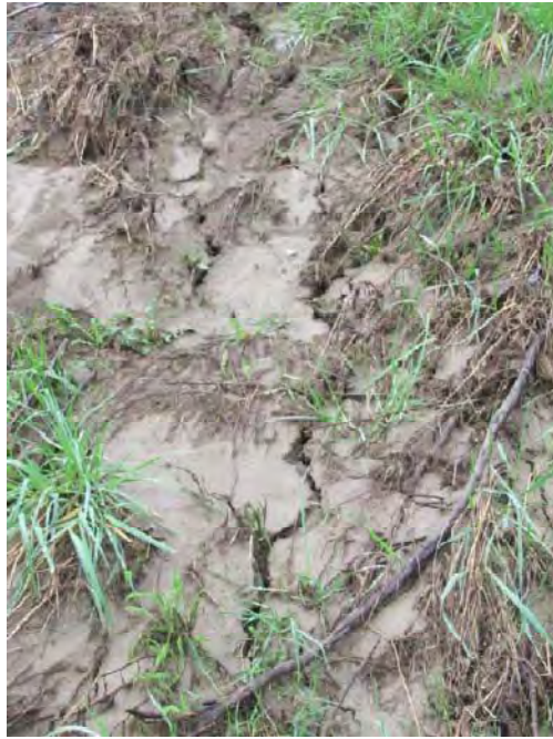
Figure 4.37 Ground damage adjacent to the bank of the Selwyn tributary near the end of Gillanders Rd (Darfield side). (Position marked as Photo 1 in Fig. 4.36; -43.596667°, 172.080000°)
