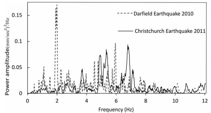
**Figure 6** Seismograms in the frequency domain for Darfield and Christchurch earthquakes at LPCC site. This record is for the east–west component of ground motion. Power spectra analyses were performed using SeismoSignal 4.3.0.
