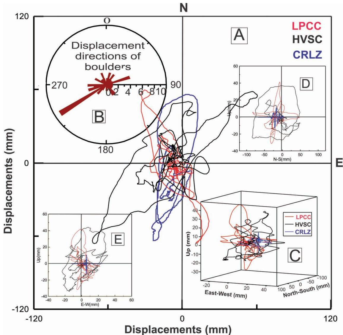
**Figure 4** A comparison of observed and instrumentally recorded displacement directions. **A**, Horizontal displacement records of three seismic stations (LPCC, HVSC and CRLZ) for Darfield earthquake; **B**, rose diagram shows displacement directions of boulders measured in the field; **C**, 3D diagram of displacements; **D**, sectional view (up versus north–south); and **E**, sectional view (up versus east–west).
