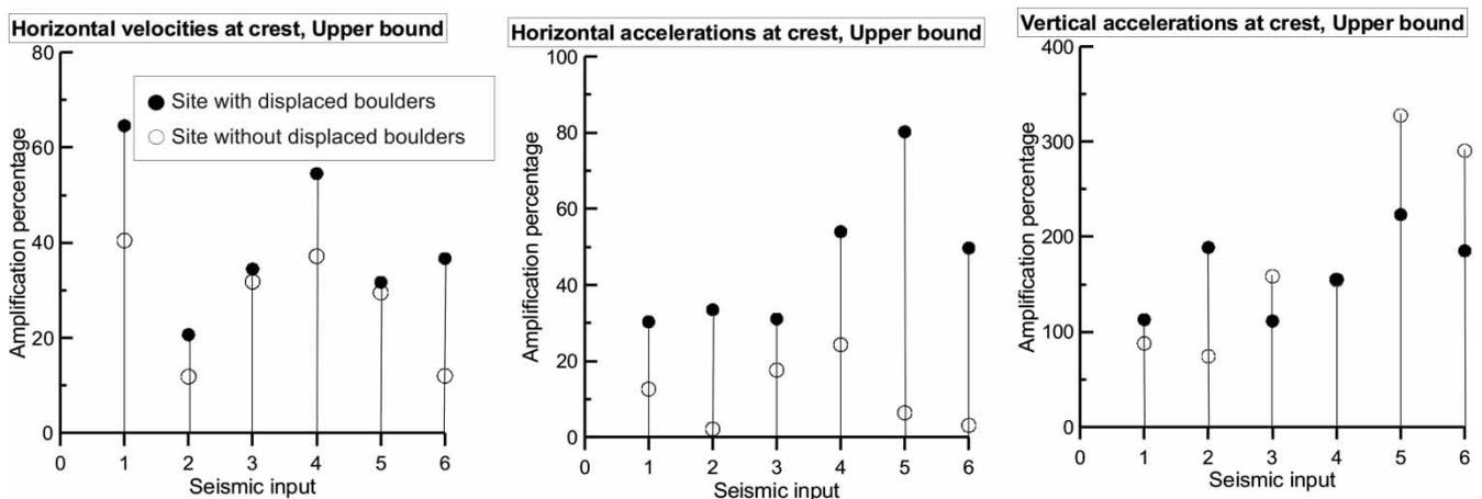
**Figure 5** Results of topographic amplification modelling along profiles AA' and BB'. Numbers 1–6 on the *x* axes show the different seismic inputs. 1, 2: LPCC data of S80W and N10W components recorded for the Darfield earthquake; 3, 4: CRLZ data of east and north components for the same earthquake; 5, 6: LPCC data of similar components recorded for the Christchurch earthquake.
