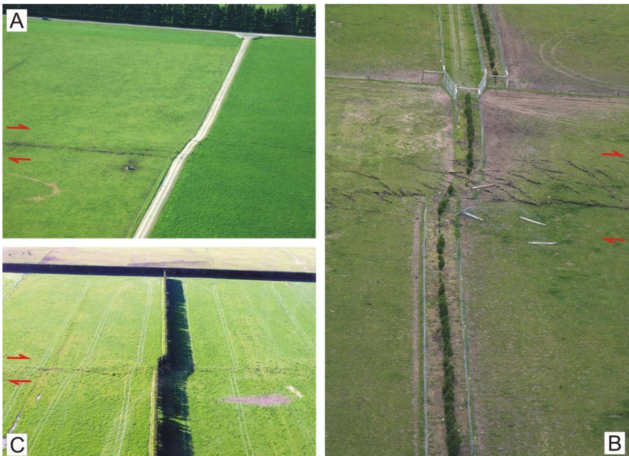
Figure 2: Oblique aerial photographs of Greendale Fault surface rupture (see Figures 1C & 1D for locations). Lateral displacement is distributed across a deformation zone of several tens of metres width; red arrows indicate relative sense of lateral displacement. A) 4.5 to 5 m of dextral displacement of a single-lane gravel road. Photo taken by Simon Cox about 11 hours after the earthquake looking north. B) ~3.5 m of dextral displacement of two wire fences and a row of small pine trees. Photo taken by Richard Cosgrove several days after the earthquake looking north. C) 4.5 to 5 m of dextral displacement of a hedge-row (wind break) of pine trees and tractor tyre tracks. Photo taken by David Barrell about 11 hours after the earthquake looking north.
