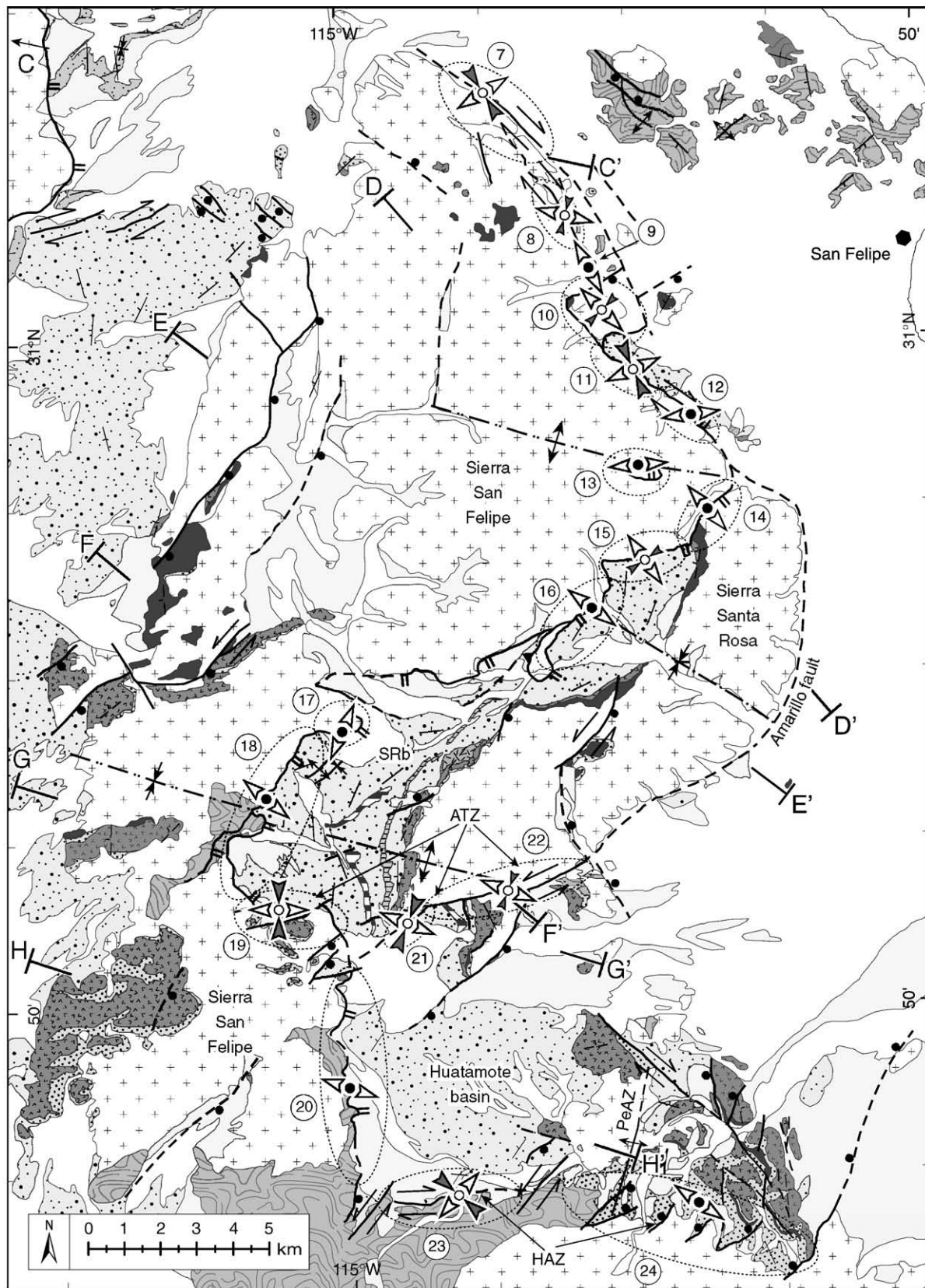
Fig. 10. Geological map of the central Sierra San Felipe and the Sierra Santa Rosa (simplified from Gastil et al., 1975; Bryant, 1986, this study) showing the trace of the Santa Rosa and Huatamote detachments. The fault curvature is thought to represent extension-parallel folding caused by N–S shortening, resulting in syn- and antiformal megamullions (inward and outward pointing arrows) in the footwall (double-dotted lines) and hanging wall (single-dotted lines) of the detachment. Stereographic projections depict fault-slip measurements showing both strike-slip and dip-slip kinematics, with arrowheads indicating the quality of the datum (see caption of Fig. 4). Local stress heterogeneities due to the fault interaction between a transfer fault (segment 19) and the low-angle detachment (segment 18) are thought to have produced atypical ENE–WSW striking dextral faults (dashed great circles in stereoplot 19). Paleostress orientations are shown with compression directions as black circles, intermediate axes as grey squares, and extension directions (trend) marked by triangles (black arrows). Faults are dashed where inferred. ATZ = Amarillas transfer zone, HAZ = Huatamote accommodation zone, PeAZ = Percebu accommodation zone, and SRb = Santa Rosa basin.
