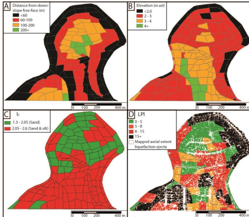
Figure 3: A) Distance of each polygon to the closest downslope free-face. B) Average elevation of each polygon. C) The average  $I_c$  for each polygon as derived from post-CES CPTu. D) The average LPI of each polygon overlain with the mapped aerial extent of liquefaction ejecta.
