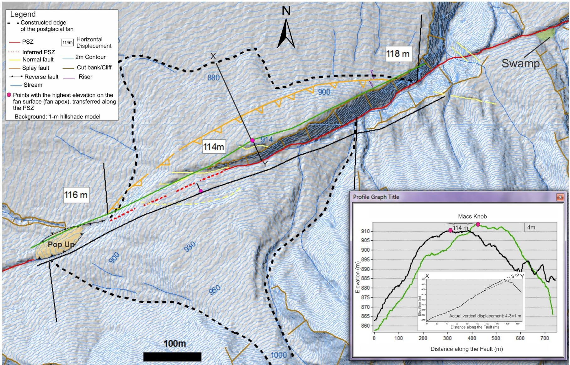
Comparing apparent trench displacements with large scale fault geomorphology to determine slip kinematics and slip rate
