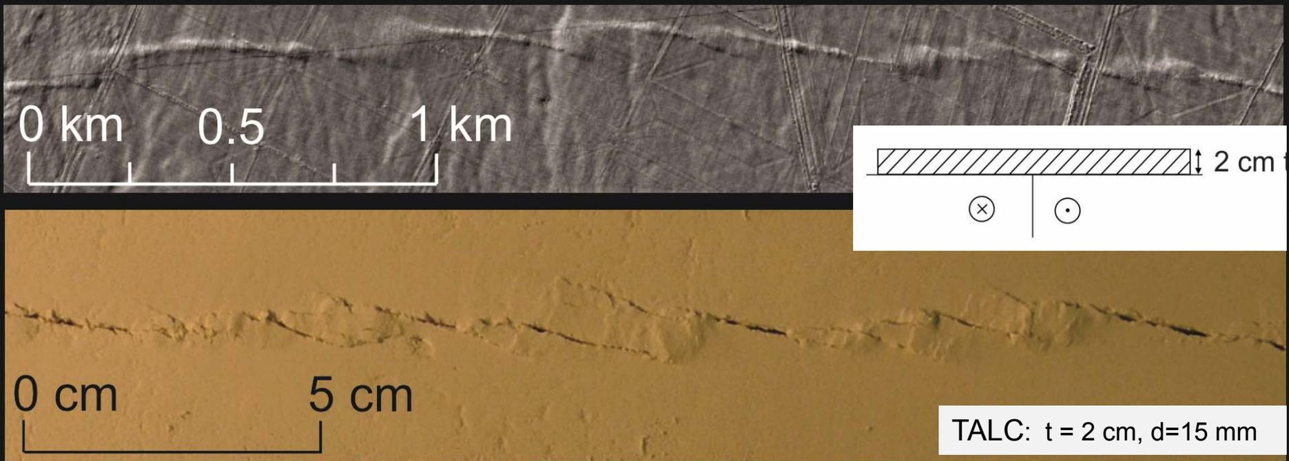
Single layer, cohesive material (talc) best replicates km-scale surface rupture morphology
