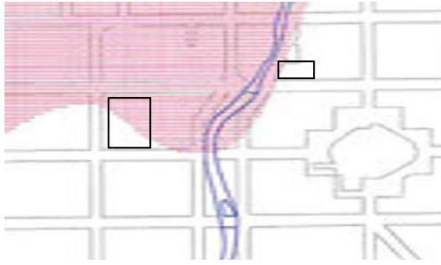
Fig. 17: Shallow liquefaction zones (~1.2 to 3m depth) beneath the Art Gallery and City Library.
