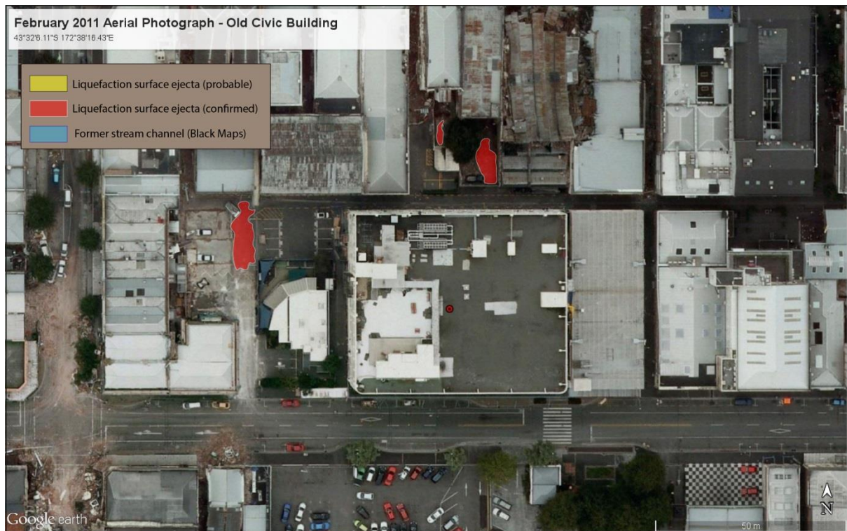
Figure 14: Map of liquefaction surface ejecta surrounding the Old Civic Building following the 22 February 2011 Mw 6.2 Christchurch earthquake
