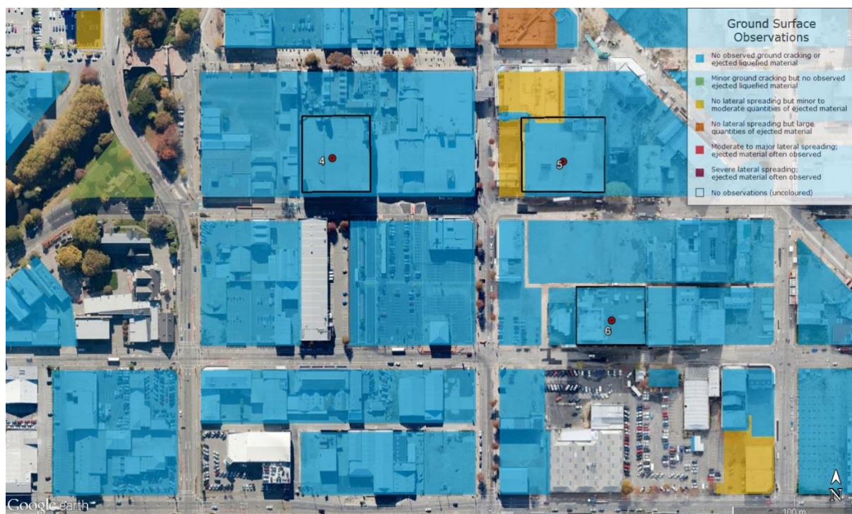
Figure 2: Area reconnaissance mapping of liquefaction and lateral spreading in the vicinity of Litchfield St carpark (4), Old Bus Exchange (5), and Old Civic Building (6) following the 22 Feb 2011
