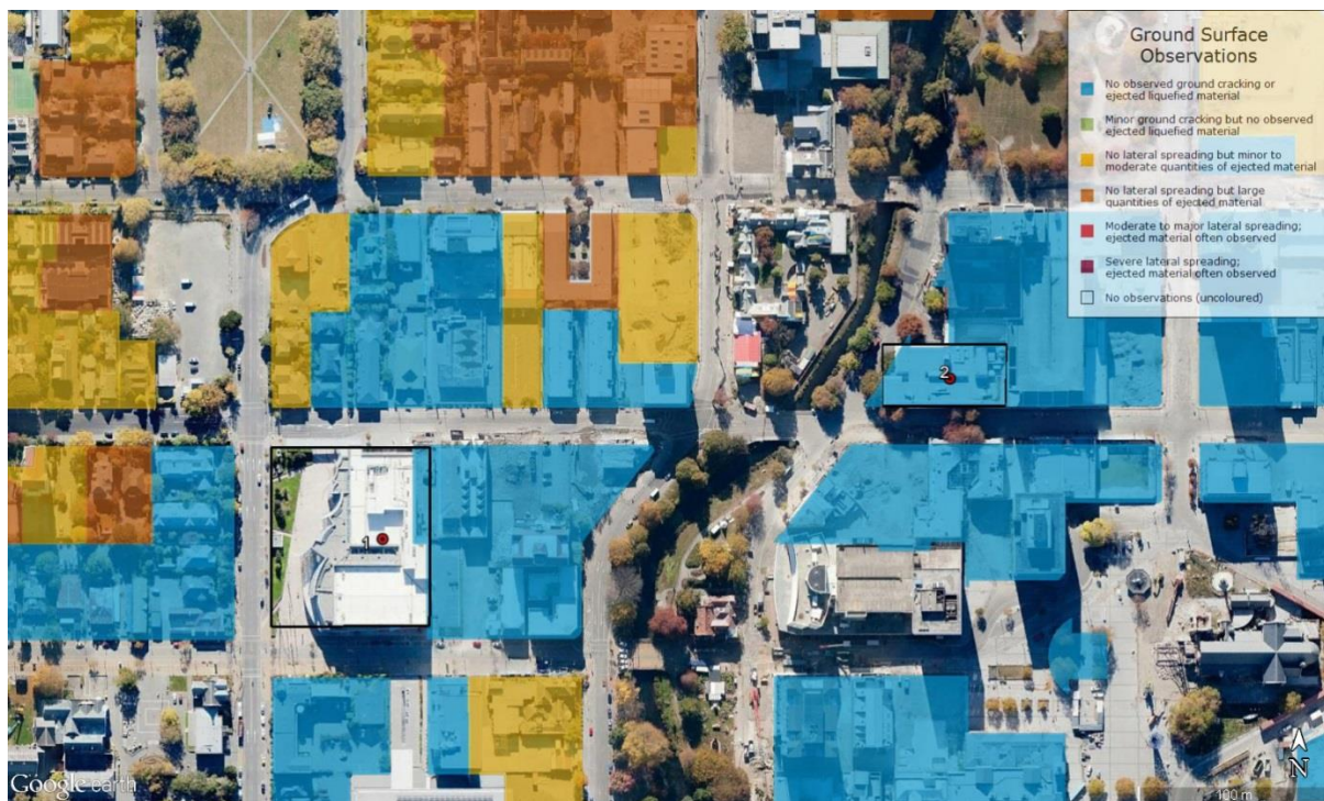
Figure 2: Area reconnaissance mapping of liquefaction and lateral spreading in the vicinity of the Christchurch Art Gallery (1) and City Library (2) following the 22 Feb 2011 Christchurch Mw 6.2
