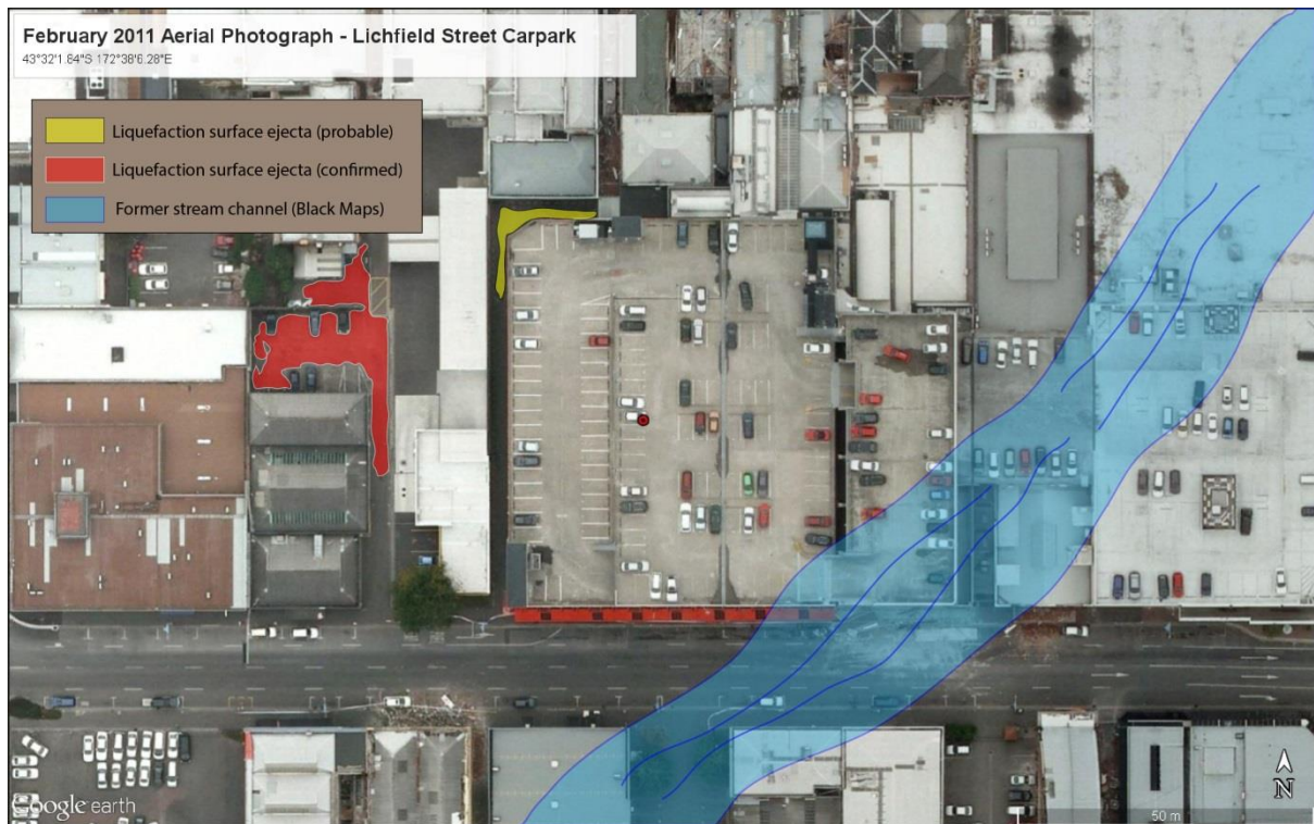
Figure 12: Map of liquefaction surface ejecta surrounding Lichfield Car Park following the 22 February 2011 Mw 6.2 Christchurch earthquake. Position of waterway identified from Black Maps as shown.
