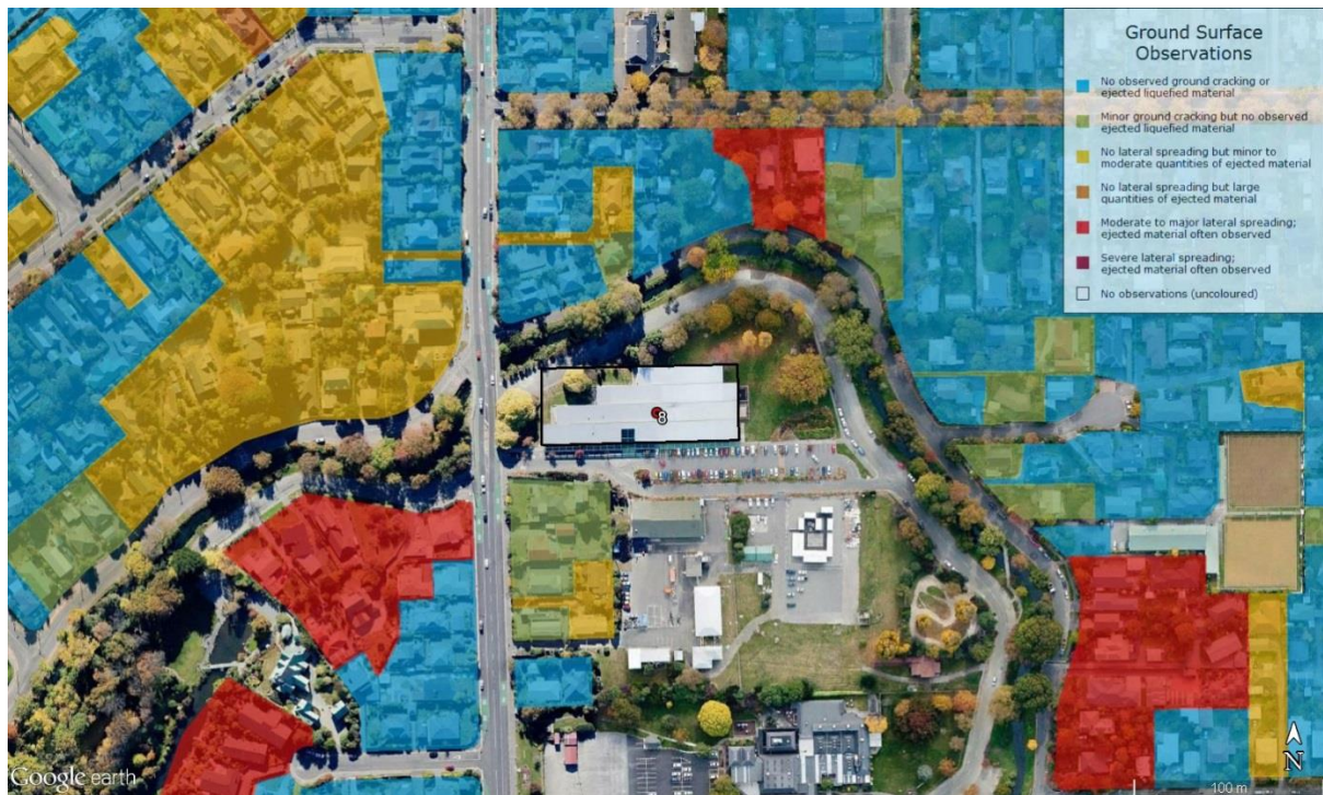
Figure 2: Area reconnaissance mapping of liquefaction and lateral spreading in the vicinity of Christchurch South Library following the 22 Feb 2011 Christchurch Mw 6.2 earthquake (mapping by Tonkin and Taylor Ltd). More detailed mapping (this report) is presented in Fig. 11
