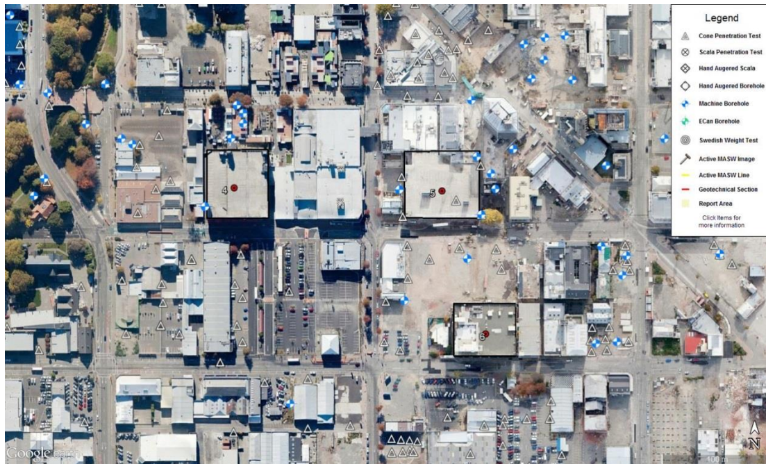
Figure 3: Location of CPT, borehole, and other geotechnical sampling sites in the vicinity of the Lichfield St carpark (4), Old Bus Exchange (5), and Old Civic Building (6). These data were variably used to construct geologic cross-sections (e.g., Fig. 10).
