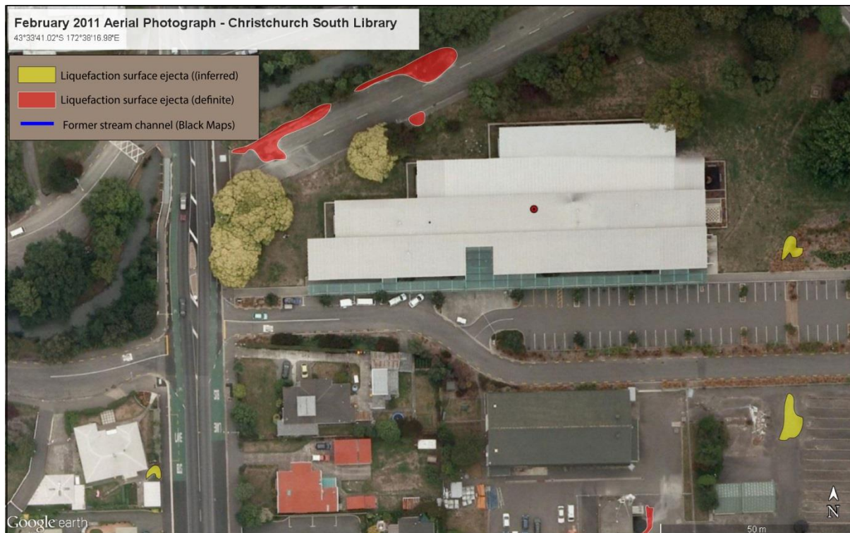
Figure 7: Map of liquefaction surface ejecta in the Christchurch South Library area following the 22 February 2011 Mw 6.2 Christchurch earthquake.
