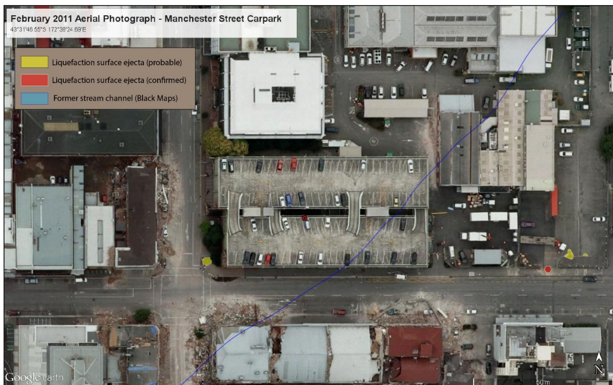
Figure 12: Map of liquefaction surface ejecta in the Manchester St Carpark site following the 22 February 2011 Mw 6.2 Christchurch earthquake.
