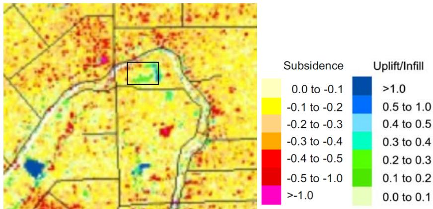
Figure 5: Permanent vertical land displacements from 2003 to December 2011 in metres for the Christchurch South Library area. Image from Hughes et al. (2015)
