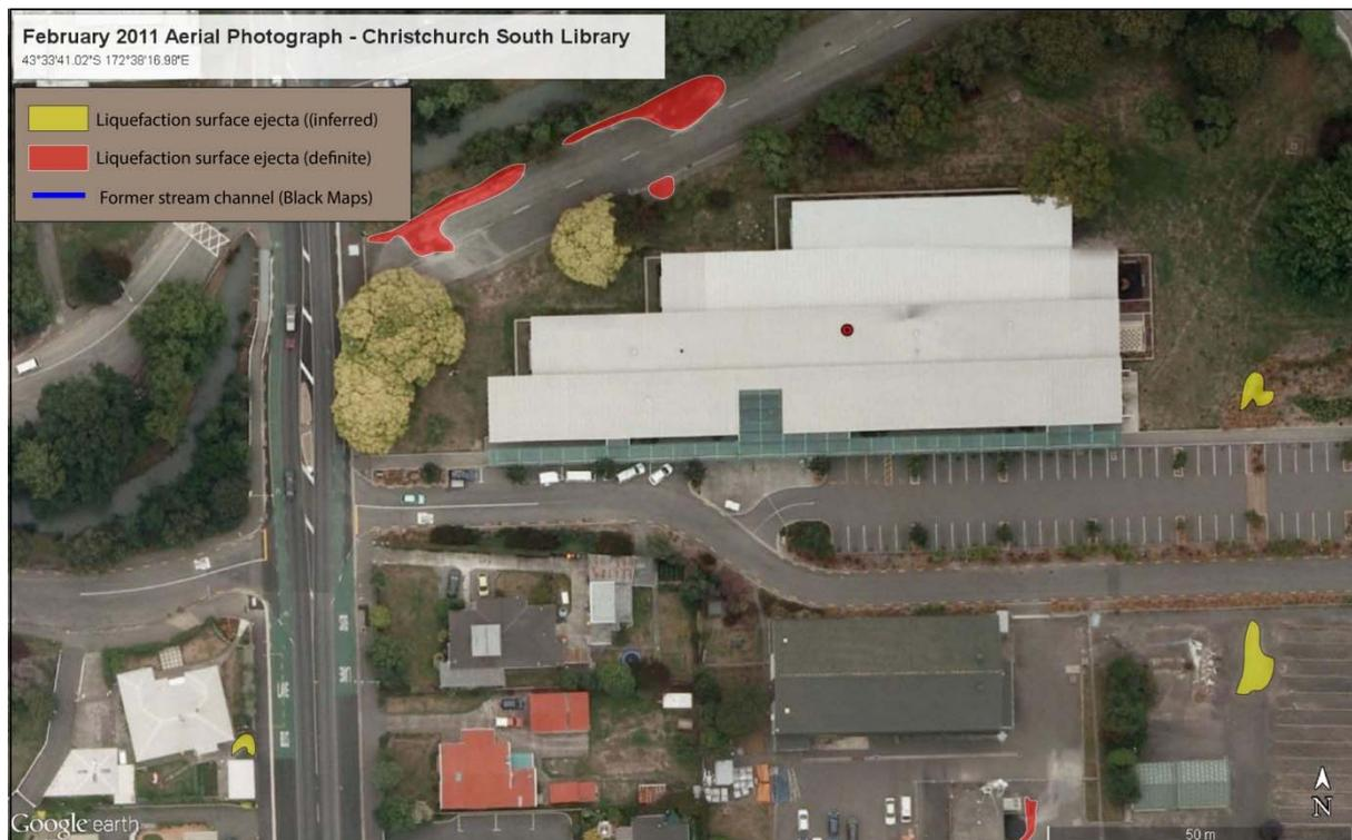
*Figure 7: Map of liquefaction surface ejecta in the Christchurch South Library area following the 22 February 2011 Mw 6.2 Christchurch earthquake.*
